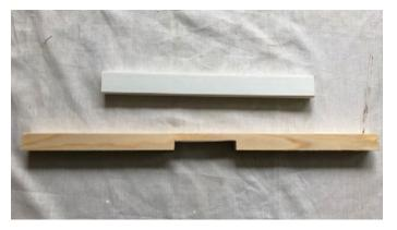
• Separate the two parts of the trunking. Starting from the middle, drill three rows of holes in the lid using a 2.5mm drill bit. They should be approximately 5mm apart and extend for 50mm (25mm either side of centre).
