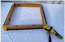
There are other clamps available that will do the job but, if you haven't got any, then assemble one side at a time without driving the nails fully home. Once complete, check for square then drive the nails home. A simple clamp can be made with any strong cord or rope but cannot be relied on to be square.
