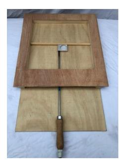
Note that the larger piece of ply extends beyond the 'box'. Without this, the weight of the handle and cable tends to tilt the hot plate risking spillage of the soda crystals and contact with the mesh floors.
