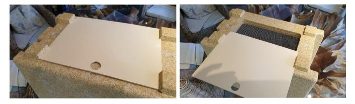
In each of the 4 feet, using a sharp modelling knife cut a groove with a height 'X' equal to the thickness of the board you intend to use for the floor.
